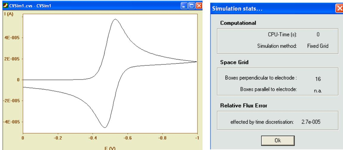
The picture on the right-hand side shows a summary of the simulation stats obtained when clicking on the **Simulation -> Stats** command:
