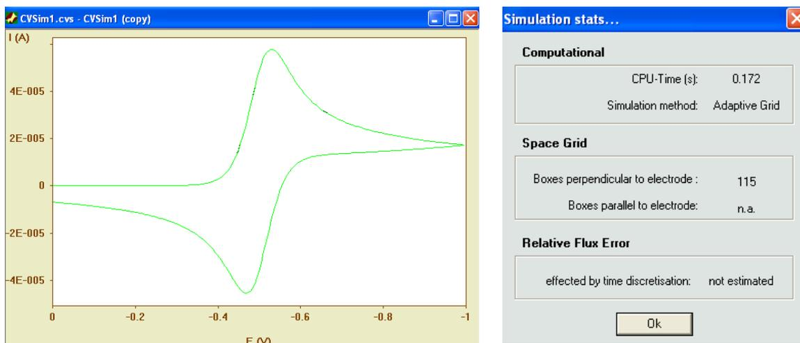
Because of *Local FEM Error* > 0 the adaptive grid refinement was enabled now. About 100 additional grid points have been introduced in the course of the simulation and the current curve converges exactly to that obtained with the box method on the 16-points grid.
