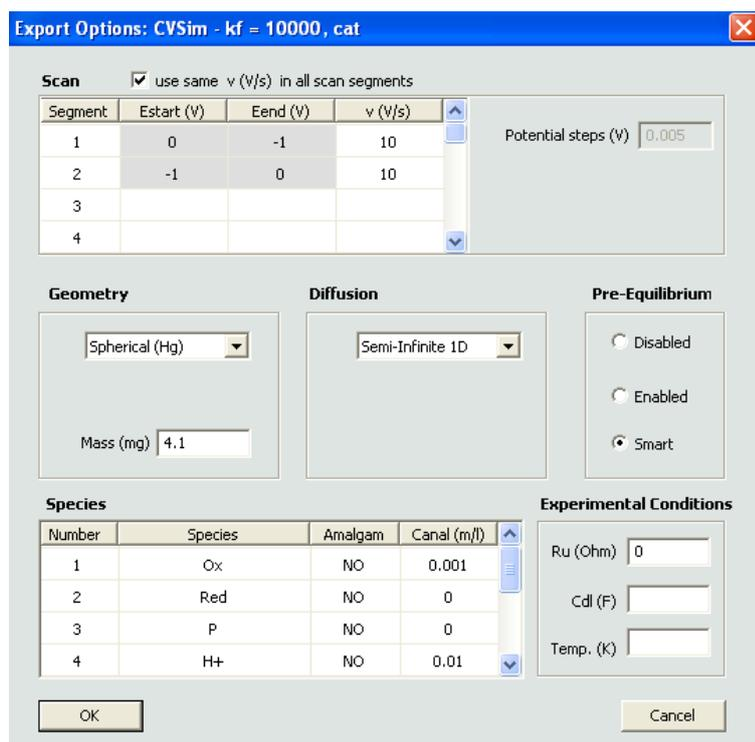
Note the difference between an empty input field and an input field where "0" has been entered. In the example shown left no entry is produced in the use-file for the double layer capacity,  $Cdl (F)$ , and for the temperature,  $Temp.(K)$ , while  $Ru (Ohm) = 0$  is explicitly written to the file.
