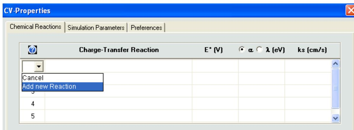
Select **Add new Reaction** and complete the appearing charge-transfer reaction template
